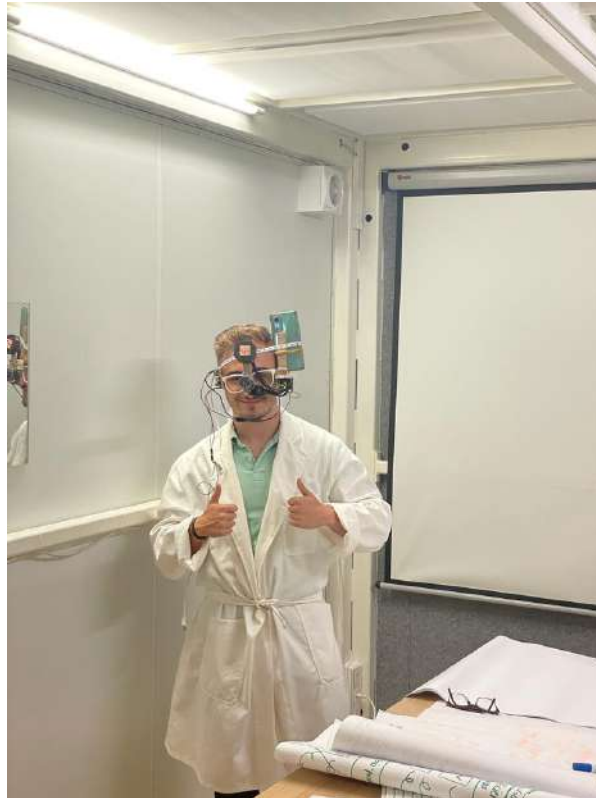
FIGURE 10. THE PROTOTYPE IN USE: THE DENTIST WOULD SIMPLY PUT ON THE GLASSES AND COULD PERFORM HIS TASKS. IN THE FINAL PRODUCT, THERE WOULD BE NO PHONE, BUT A PROFESSIONAL CAMERA.
