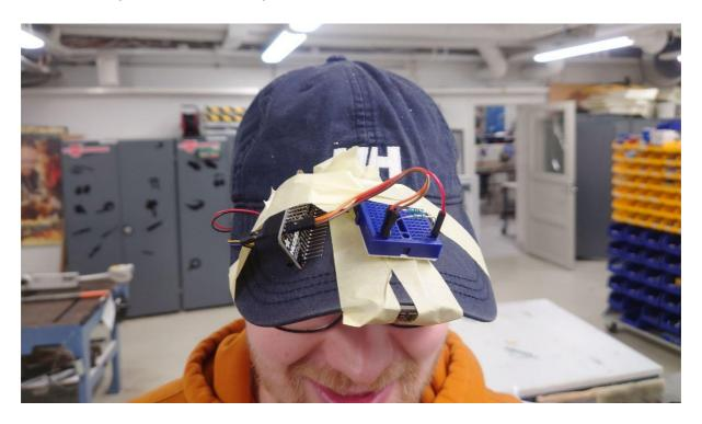
The device is meant to be used by personnel to monitor the work environment. Firstly, the device can monitor ways of working if required to respond to specific company policy. This could be useful in dangerous or volatile working environments. The lens' ability to focus will keep the device small. Secondly, the device can also monitor the temperature and moisture levels of the work environment to ensure a healthy workplace.
