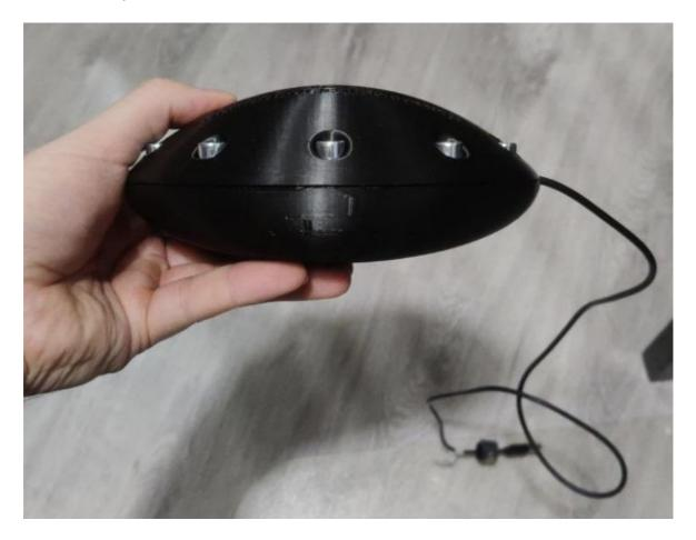
The device is a prototype to observe environments and capture air measurements from a drone. While the drone camera can be used for navigation the IALL lens allows for a broader range of focus for image or video capturing.
