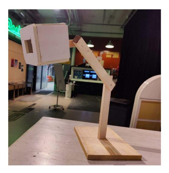
The system was designed as a prototype for astrophotography and videography and would be placed on the top of the hill. The concept features 3 degrees of freedom to help the lens change its orientation.
