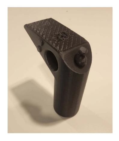
During planning the team identified the positioning of buttons on only one side as a possible challenge to persons who are not right-handed. One solution included buttons on both sides, allowing the user to activate the side they prefer. As this could potentially lead to accidental button activation when swopping between users, a joystick option usable by both left-and-right handed users was incorporated.
