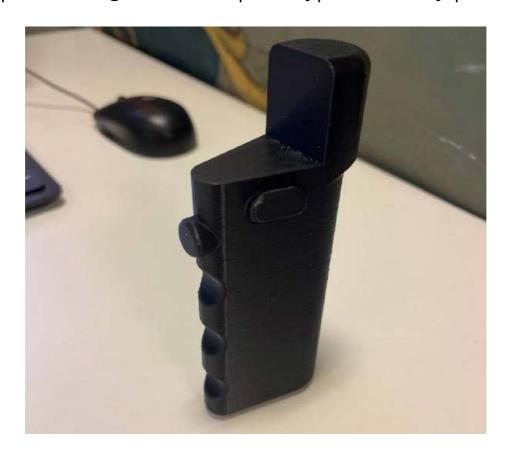
The final prototype opted for a button positioned on the inside of the user's grip, allowing one to depress the button with the middle section of an index finger, while the index fingertip is positioned to depress the second button.
