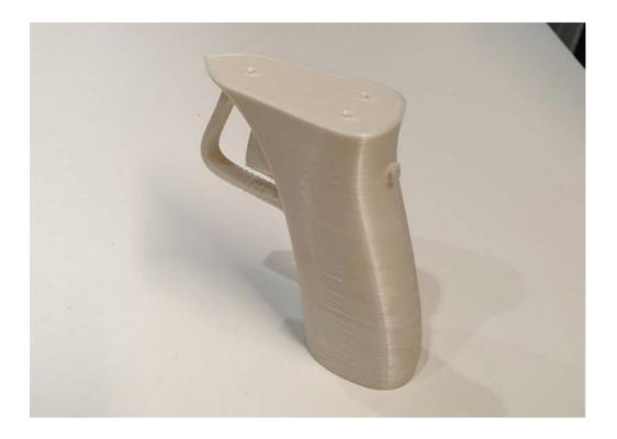
After all team members tested the clay version of the prototype the handle was shaped to follow the curve of one's hand and the second button was relocated to the back of the handle for increased accessibility.
