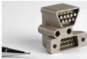
Figure 16 : Image of the feedthrough KET brick (AJP version) casted with epoxy
