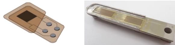
Figure 17: 3D view of a AJP RTD sensor (left) and image of a RTD sensor and a heater deposited on a 316L substrate (right)
