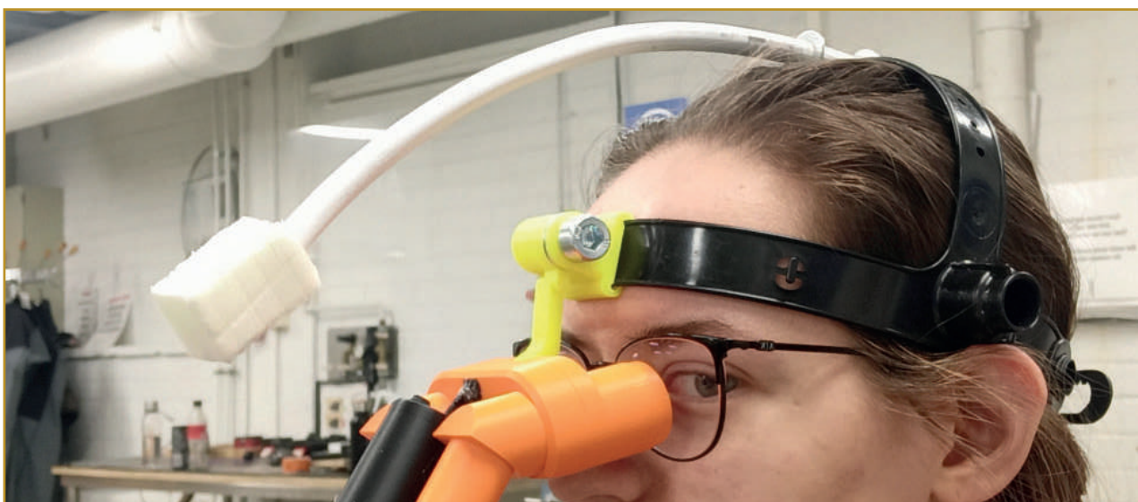
Figure 21: Flexible cable light mounts onto the headband instead of the headset.
