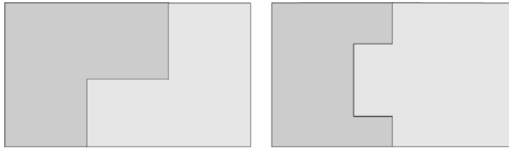
Figure 26. Dividing line for the box, as the drawings (left) and as produced (right).
