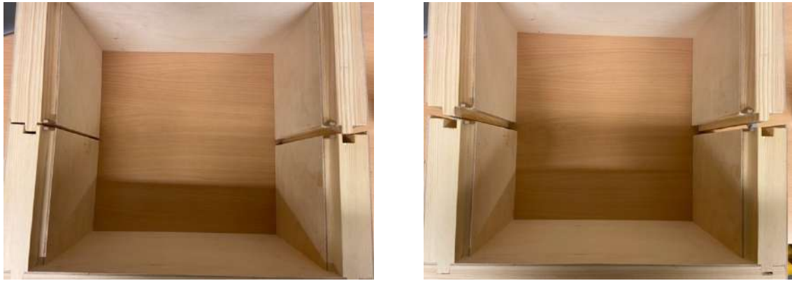
Figure 39: The opening when separating the box by bending the hoops in the eccentric locks unevenly (left) versus evenly (right).
