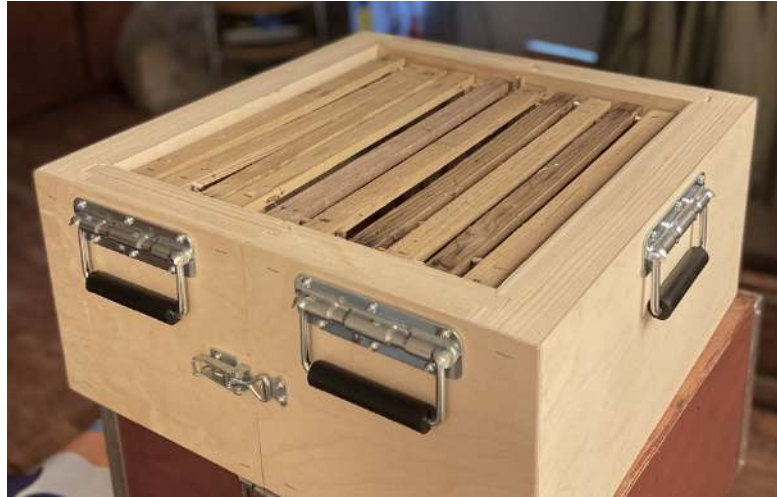
Figure 38: A picture of the prototype box filled with ten empty honey frames to illustrate the fitting of the frames and that the mounted stops create a desired spacing between the frames.
