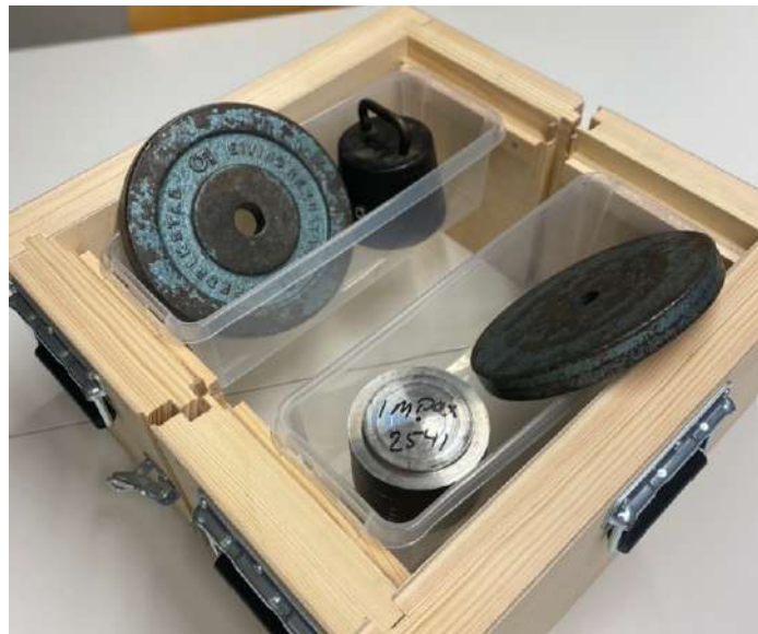
Figure 29: A picture of the build prototype of the dividable box prepared for the tests. The weights correspond to the weight of ten honey filled frames.
