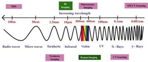
Figure 2 Wavelenghts for different imaging technologies (Source: (Gautam et al., 2015))
