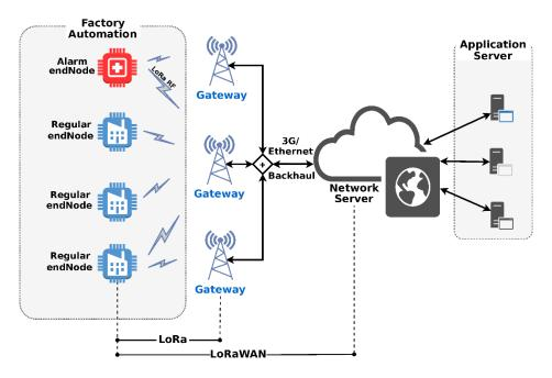
Figure 24 System LoRaWAN (Source: (Filho et al., 2020))
