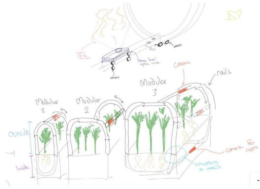
Figure 18: Moving camera system for aeroponic plants (Scribble by Linnea Seeskari)
