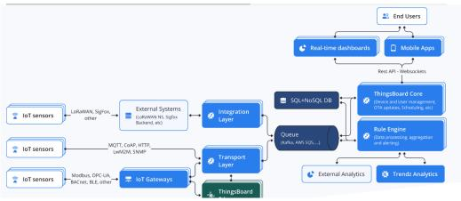
Figure 22 IoT System Architecture Thingsboard for the use case of smart farming (Source: (Thingsboard, n.d.))
