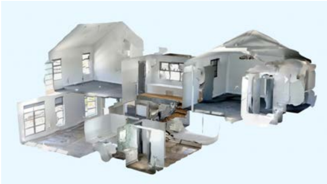
Figure 16: 3D map of a house using a LIDAR scanner and a camera in sync. Source: Polycam
