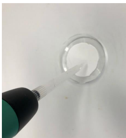
Figure 19: Casting of CNF on Whatman Filter
