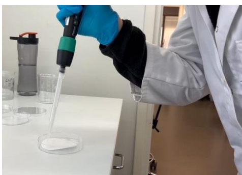
Figure 18: Casting Process of films
