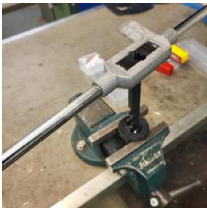
Figure 29: Threading process of a 12mm hole for the lens holding part of the camera
