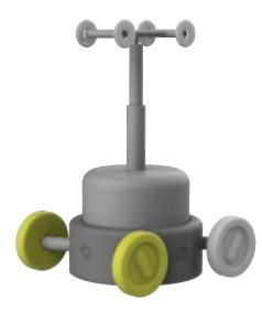
Our chosen navigation solution uses a motorized support arm that stretches from the robot to the opposite pipe wall. This approach provides several key advantages: the stabilizing arm ensures the robot remains securely in place, even under high water pressure and turbulent flow conditions. Additionally, this method offers precise control over the robot's movement and position, which is crucial for navigating complex pipe networks and ensuring the successful deployment of the sealing mechanism.
