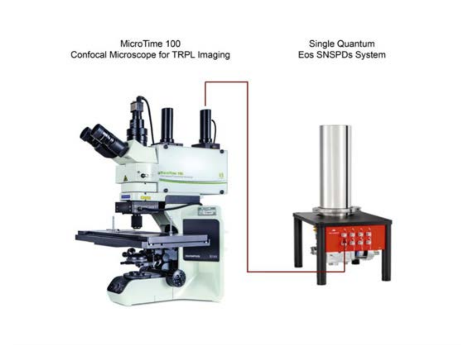
Figure 3. MicroTime 100 Confocal Microscope with SNSPDs coupling (PicoQuant GmbH, n.d.).
