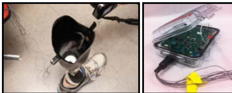
The portable device tracks how much a person's limb swells and shrinks when inside a prosthetic socket. Joan Sanders, U of Wash.
