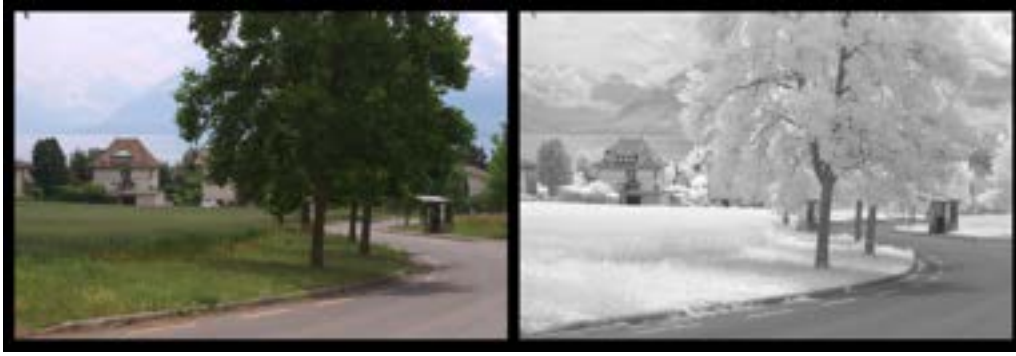
Figure 5: Comparison between RGB Imaging (right) and NIR Imaging (left)
